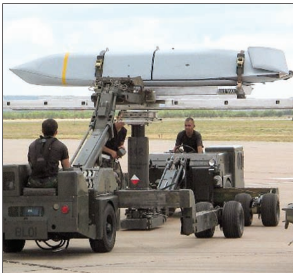
The AGM-158 stealth cruise missile—manufactured by defense contractor Lockheed Martin—shows a sleek, white profile. It is about 14 feet long and weighs approximately 2,250 pounds. Was this what several witnesses say they saw flying low over the ground near Shanksville, Pa. on Sept. 11, 2001? Above, U.S. military personnel prepare an AGM-158 for deployment.
